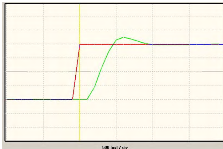
Figure 1: Current controller step response
